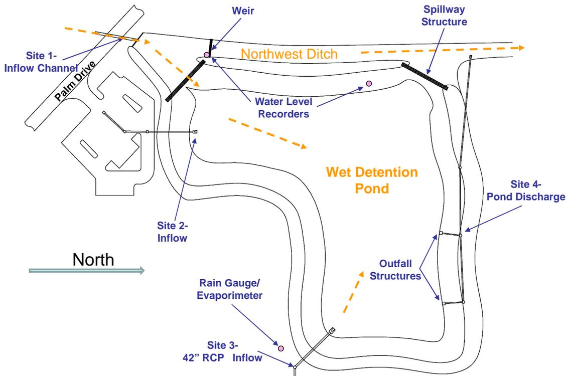
Figure 2-1. Schematic Overview of Locations for Monitoring Equipment at the Pioneer Key Regional Stormwater Facility.
