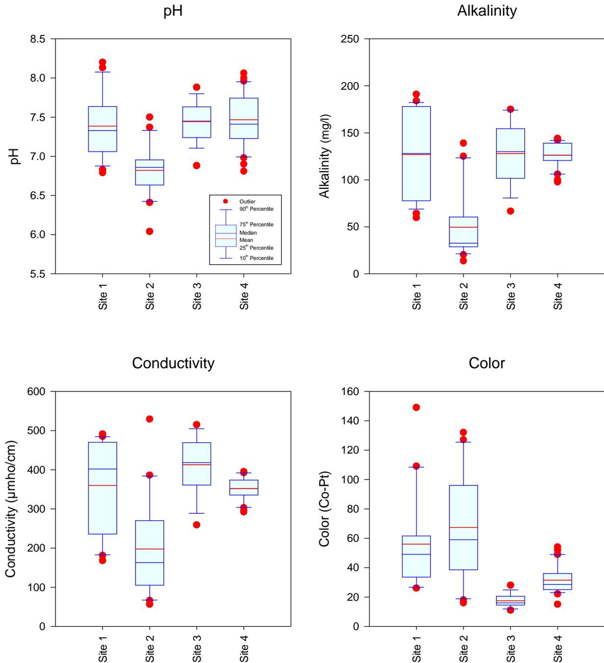
Figure 3-9. Summary of Statistical Variability in General Parameters Measured in Inflow and Outflow Samples at the Pioneer Key Wet Detention Pond Site.
