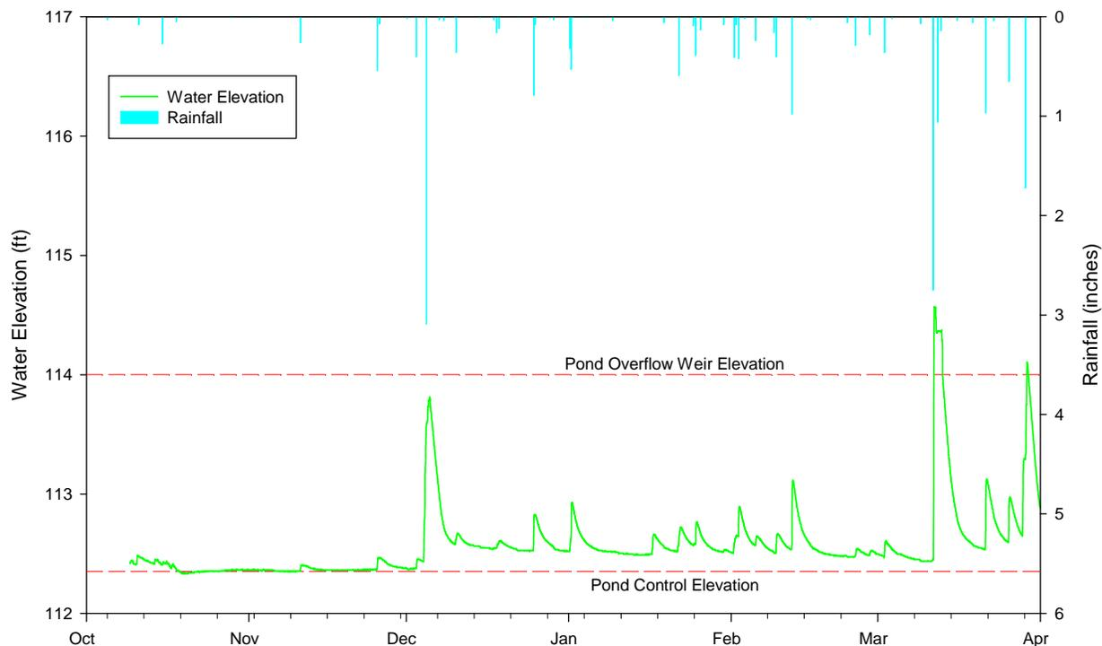
Figure 3-6. Water Surface Elevations in the Pioneer Key Pond from October 2009-March 2010.
