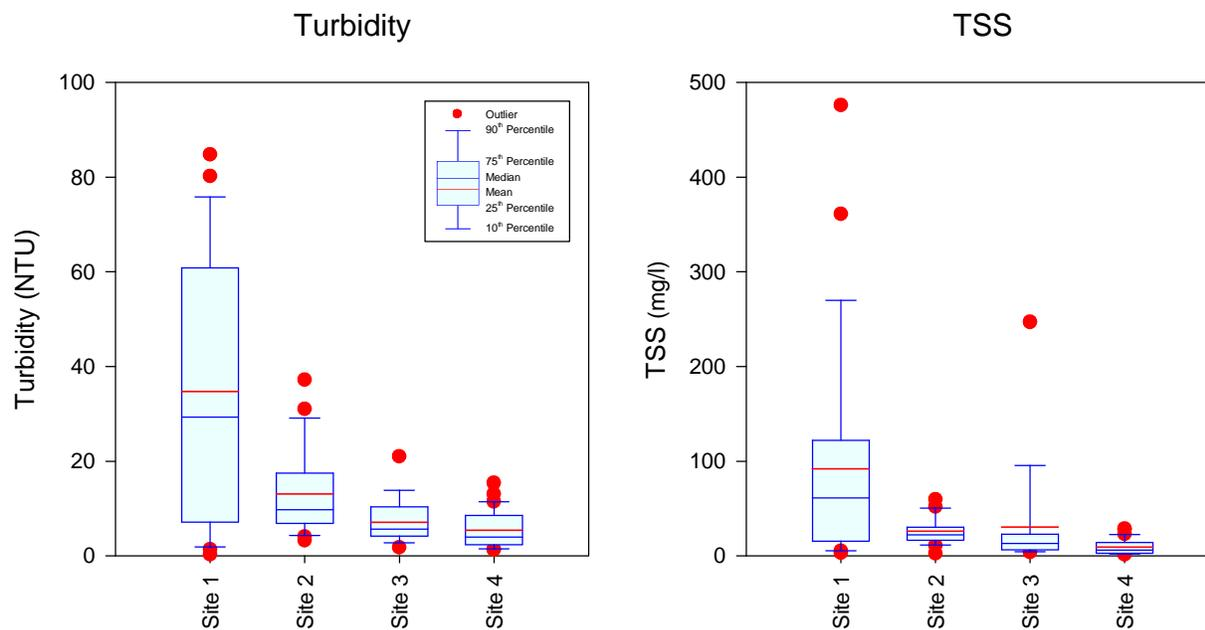
Figure 3-12. Summary of Statistical Variability in Turbidity and TSS Measured in Inflow and Outflow Samples at the Pioneer Key Wet Detention Pond Site.
