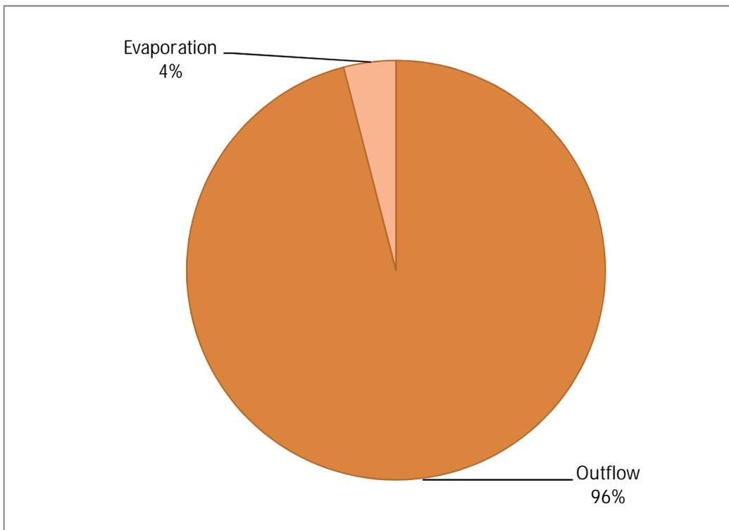
Figure 3-8. Hydrologic Inputs and Losses for the Pioneer Key Wet Detention Pond from October 2009-March 2010.
