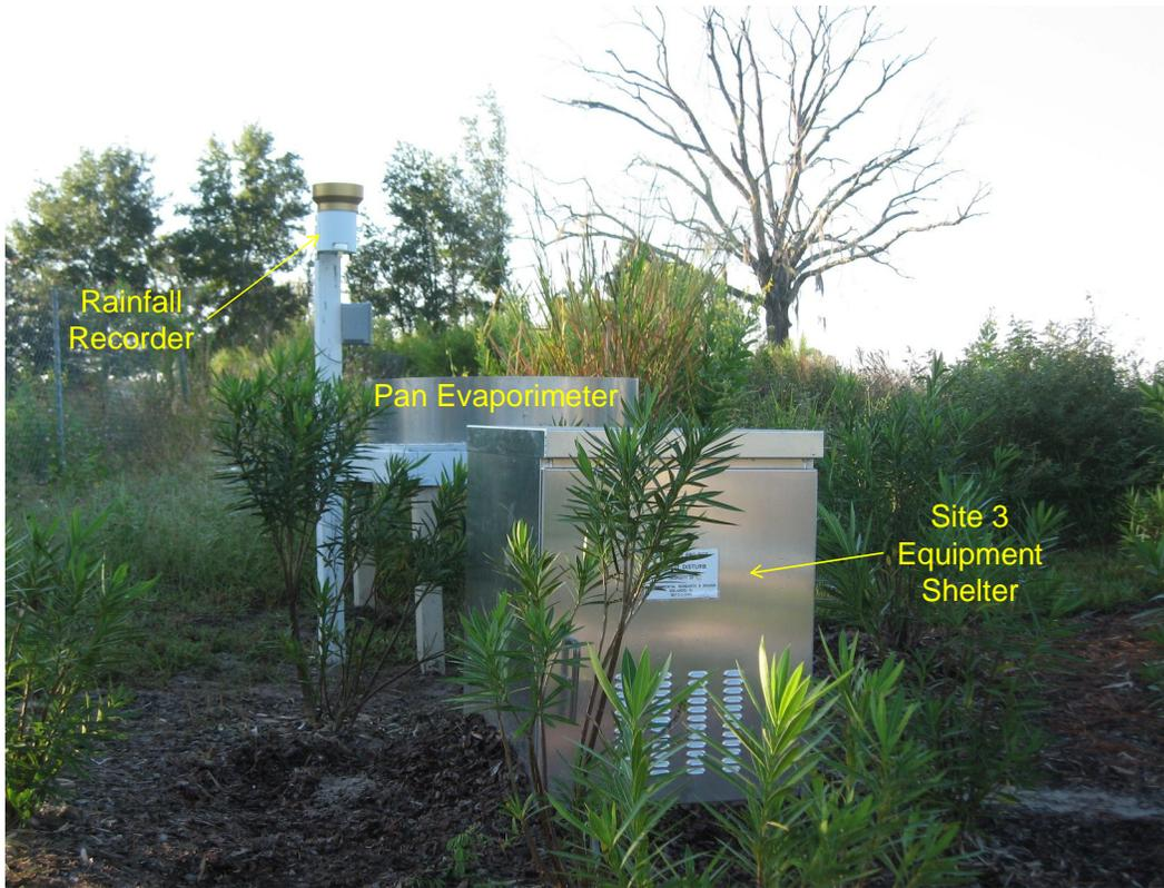
Figure 2-5. Monitoring Equipment Installed at Site 3.
