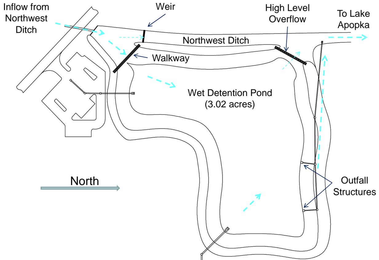
Figure 1-3. Schematic of Flow Patterns in the Pioneer Key Regional Stormwater Facility.
