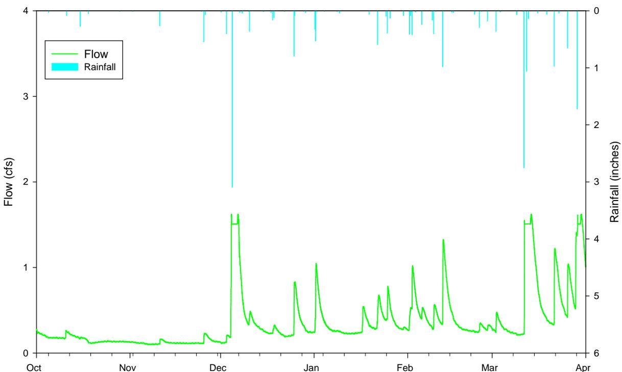
Figure 3-5. Measured Discharge Hydrographs from the Pond Outfall Structures (Site 4) from October 2009-March 2010.
