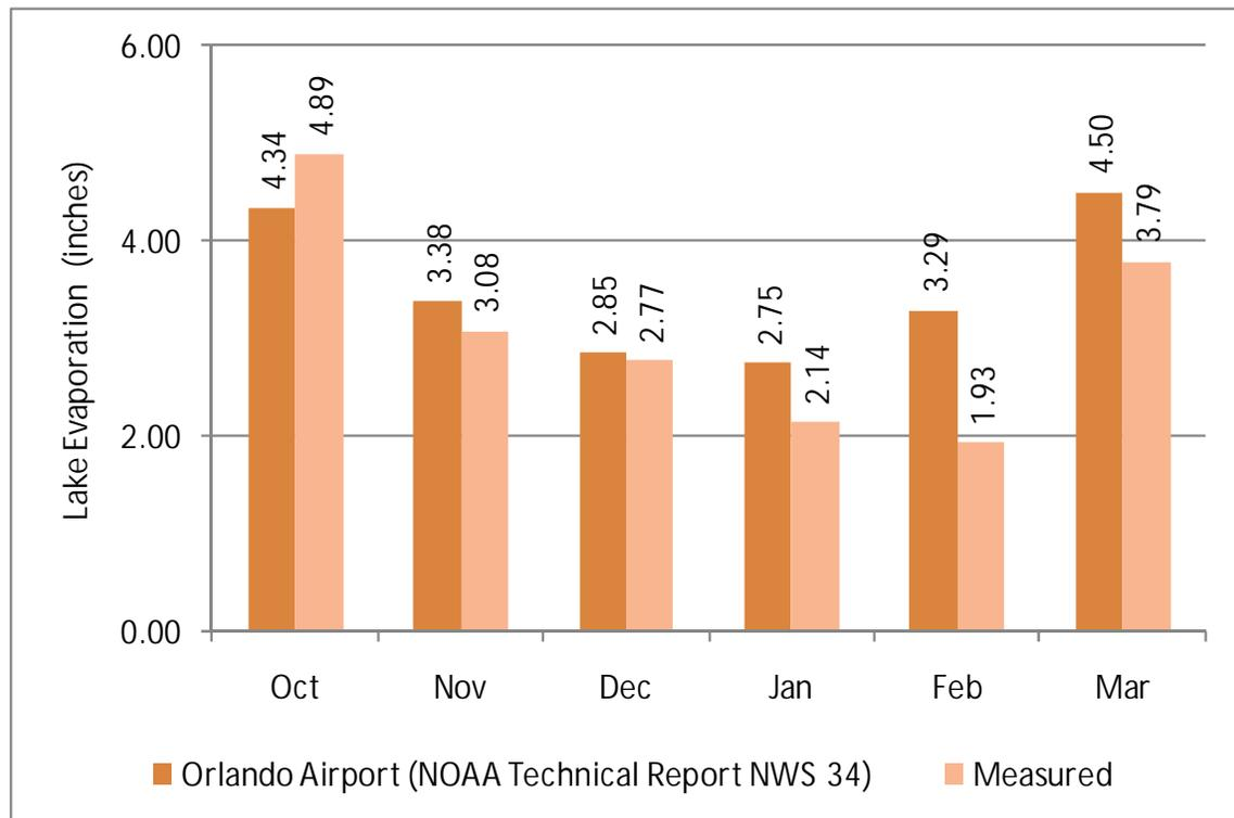
Figure 3-7. Comparison of Average and Measured Evaporation at the Pioneer Key Wet Detention Pond Site.
